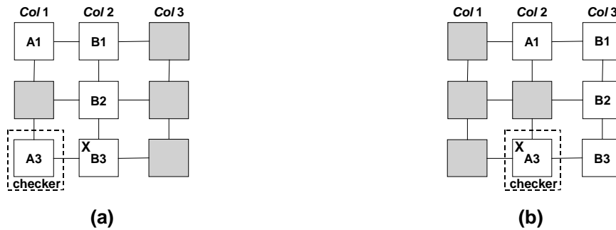
Figure 4.3: Effect of reconfiguration order. (a) Original configuration. (b) Alternative configuration when column 1 is intentionally unused.
