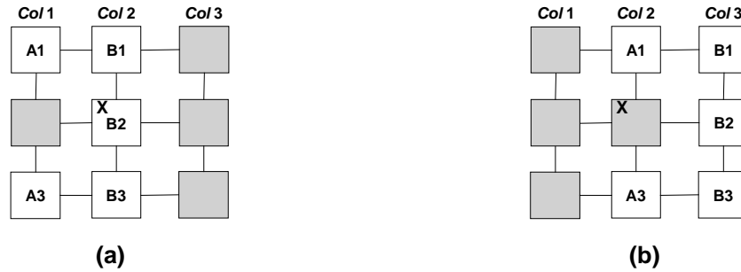
Figure 4.2: Example of undefined fault location. (a) Original configuration. (b) Alternative configuration when column 1 is intentionally unused.
